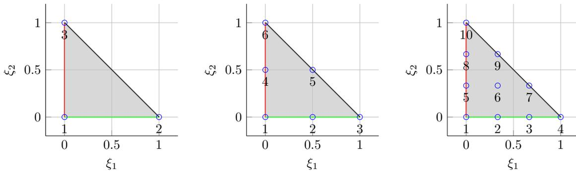
Figure 1: Triangular finite element in reference domain ( $\xi_1$ - $\xi_2$  space) with 3 nodes ( $p = 1$ ) (left), 6 nodes ( $p = 2$ ) (center), and 10 nodes ( $p = 3$ ) (right). The faces are numbered as: face 1 (—), face 2 (—), and face 3 (—).
