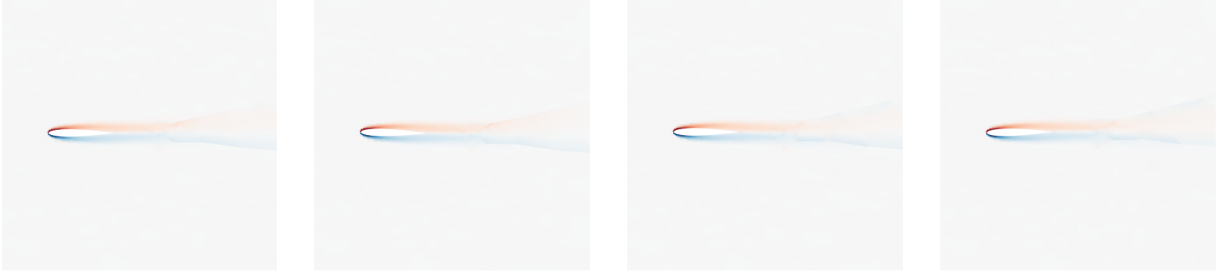
Fig. 5 Airfoil motion and flow vorticity corresponding to foil-damper system under prescribed rotational motion \theta(t) = \mu_A^{\text{init}} \cos(2\pi ft + \mu_\phi^{\text{init}}) with frequency f = 0.2 at various snapshots in time: t = T, \frac{5}{4}T, \frac{6}{4}T, \frac{7}{4}T (left-to-right, top-to-bottom).
