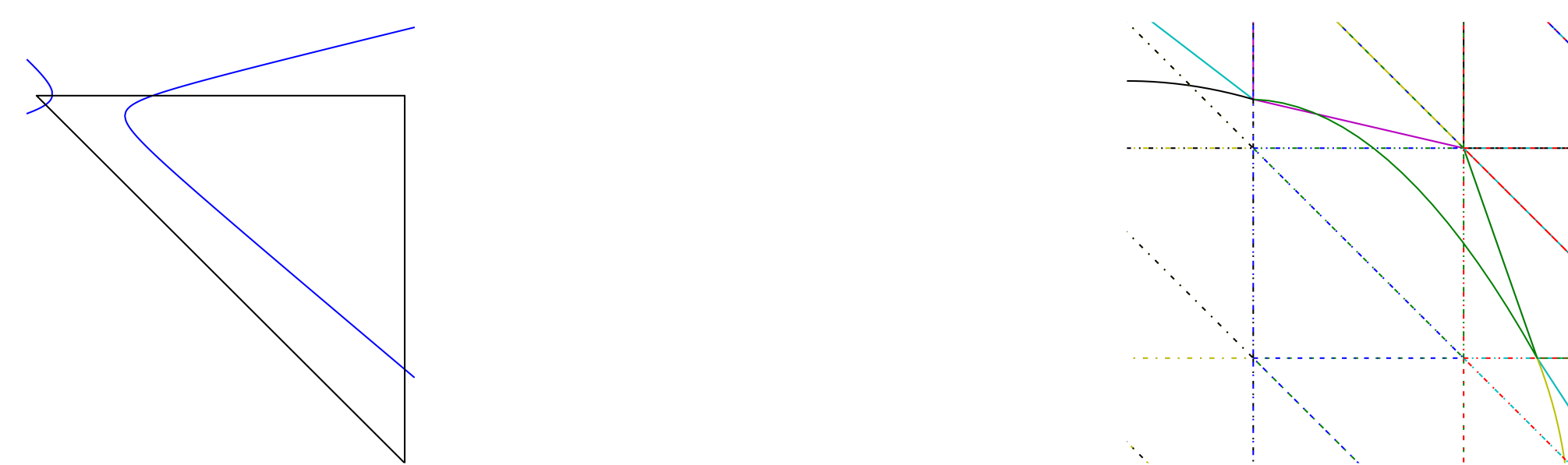
Example case to ignore (left) where the level-set function approximation intersects at four different points with an element. Example case to avoid (right) where reasonable positions at all six nodes generate an inverted element.
