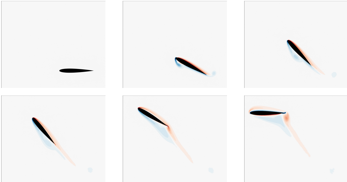
Figure D.9: Flow vorticity around airfoil undergoing motion corresponding to optimal rigid body motion, i.e., solution of (D.44) under parametrization PII ( \rightarrow\leftarrow ). This rigid body motion further reduces the degree of flow separation and required work to complete the mission. This motion differs from the solution of PI as it has a larger pitch amplitude and slightly overshoots the final vertical position before settling to the required position. Snapshots taken at times t = 0.0, 0.8, 1.6, 2.4, 3.2, 4.0 .
