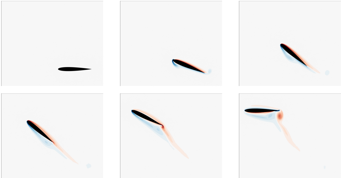
Figure D.8: Flow vorticity around airfoil undergoing motion corresponding to optimal pitching motion for fixed translational motion, i.e., solution of (D.44) under parametrization PI ( \ominus ). The pitching motion greatly reduces the degree of flow separation and vortex shedding compared to the initial guess, and requires less work to complete the mission. Snapshots taken at times t = 0.0, 0.8, 1.6, 2.4, 3.2, 4.0 .
